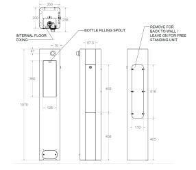
Remove rear access panel which is held on with 6 security screws. Discard panel if fixing to the rear wall - retain access panel for re-fitting later if using as a freestanding unit.
