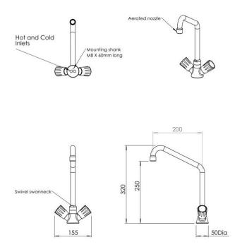
Supplied with two inlet stainless steel hoses 300mm long 3/8"BSP female connections
